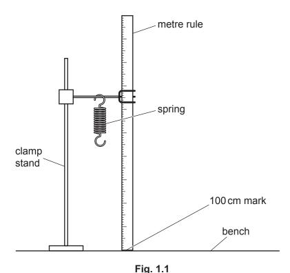
**4.** Four 20 g slotted masses with a 20 g mass hanger, each labelled 0.2 N, is ideal. If these are not available, a light hook must be provided so that loads of 0.2 N, 0.4 N, 0.6 N, 0.8 N and 1.0 N, can be suspended from the spring.
